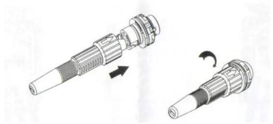
The arrow part of fiber connector is above, insert fiber connector into the socket and then rotate the arrow part clockwise
