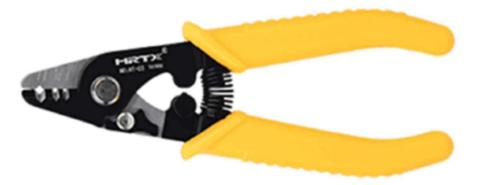
The three-hole Fiber Optic Stripper performs all common fiver stripping functions. The first hole of this Fiber Optic Stripper cuts the 1.6-3 mm fiber jacket, down to the 600-900 micron buffer coating. The second hole strips the 600-900 micron buffer coating down to the 250 micron coating. The third hole is used to strip the 250 micron fiber cable down to the 125 micron glass fiber without nicks or scratches. The handles are coated with TPR (Thermoplastic Rubber).
