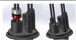
6.Put the oval ports sealing devices into the oval port and screw up the oval port.
