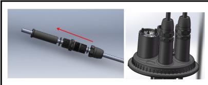
5. Put the round ports sealing devices into the round port and screw up the round port.
