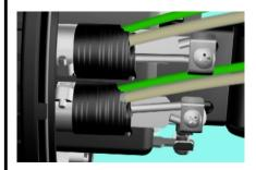
5.Fix the cable on the hose clamp and tighten the screw to fix the cable strength member.
