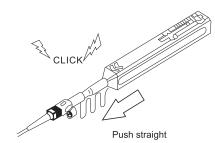
Be careful not to slant the Fiber End-Face Cleaning Pen SC while inserting into the adapter.
