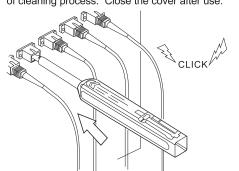
Push the Outer Shell to start cleaning the SC connector end face. A "click" sound indicates end of cleaning process. Close the cover after use.
