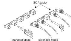
2. Insert SC connector into the Guide Cap.
