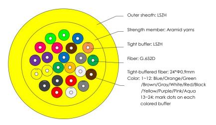
Optical fiber, tight buffer and sheath types are selected according to customer's requirements. Conventional supply types are PVC tight buffer and LSZH sheath.
