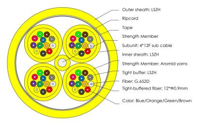
Optical fiber, tight buffer and sheath types are selected according to customer's requirements. Conventional supply types are PVC tight buffer and LSZH sheath.
