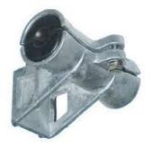
This hardware is widely used to secure ADSS cable. It has an interlocking hinge mechanism for easy insertion and securing of the cables. The clamp is secured to the pole either with a 5/8 inch through bolt (M16, not included) or with a steel band (3/4 to 1 1/4 inch). Depending on the cable diameter, there will be different dielectric pad inserts. See chart to decide appropriate part number.
