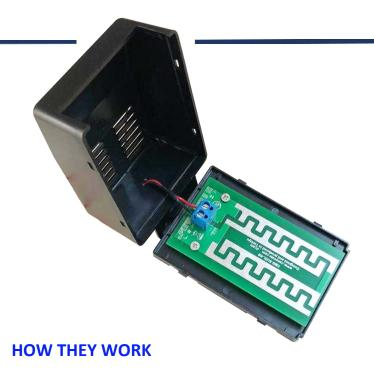
We offer basic types of float sensors that are bottom mounted. They work on the principle of short circuit between 2 copper bars.
